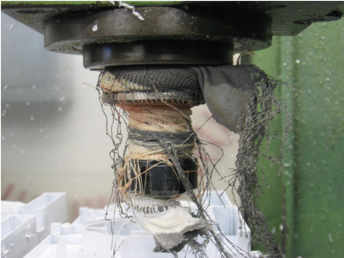
Figure 3.3.2.2: Example of clothing caught in machinery. luckily the operator was not sucked into the machine
